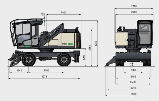
Dozer blade in addition to 4-point stabilisers
