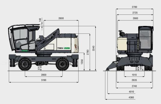
Dozer blade in addition to 4-point stabilisers
