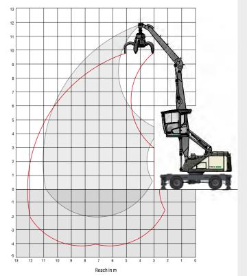
The lift capacity values are stated in metric tons (t). The pump pressure is 360 bar. In accordance with ISO 10567The lift capacity values are stated in metric tons (t). The pump pressure is 360 bar. In accordance with ISO 1052the lift capacity values represents 75% of the static tipping loads or 87% of the hydraulic lifting force (marked \*). On
