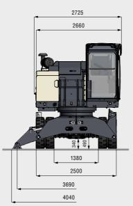
Undercarriage equipped with 2-point stabilisers and support blade
