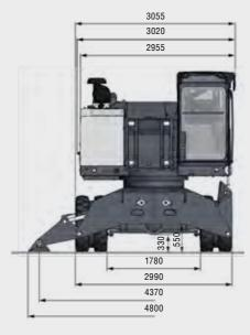
Dozer blade in addition to 4-point stabilisers
