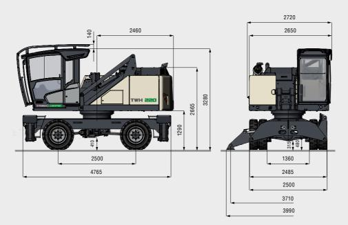
Undercarriage equipped with 2-point stabilisers and support blade
