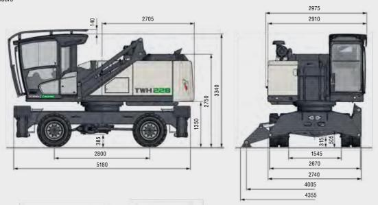
Dozer blade in addition to 4-point stabilisers
