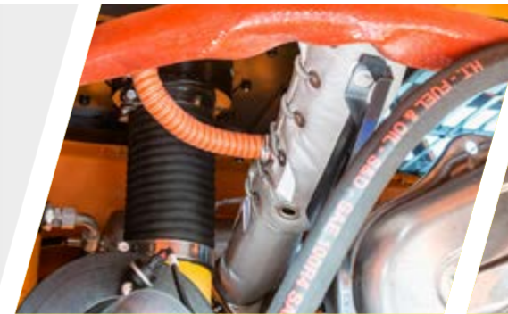
Heavy-duty filtration system (ejector)
