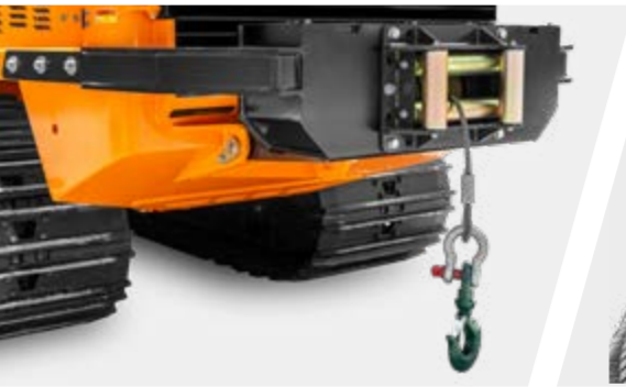
Rear winch with 13-t traction force
