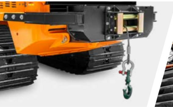
Rear winch with 6-t traction force
