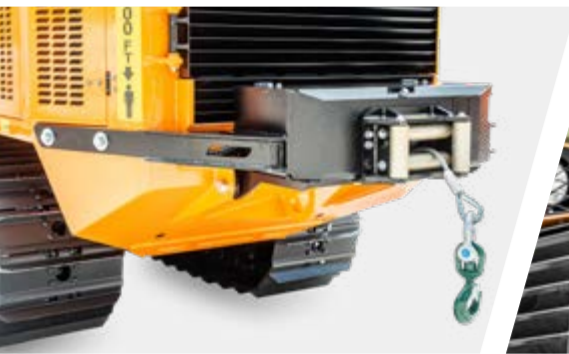
Rear winch with 6-tpulling force
