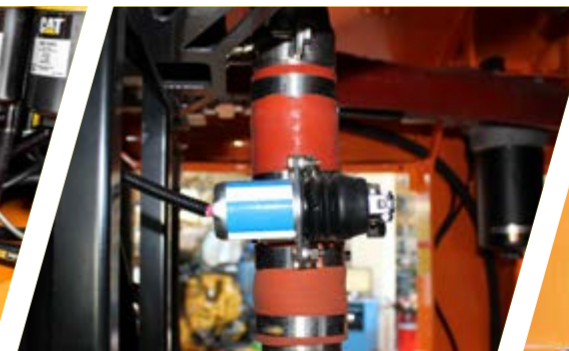
Air shut-off system
