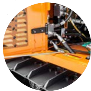
The large rear doors have safety catches (2)
