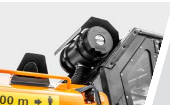
Cabin pressurization system
