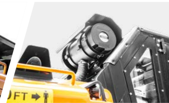
Cabin pressurization system
