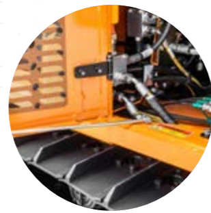
The large rear doors have safety catches (2)
