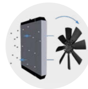
A reversible fan maximizes radiator efficiency (4)
