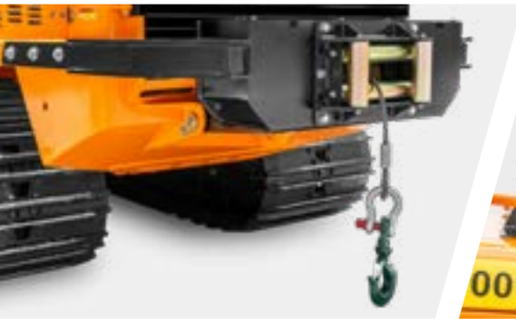
Rear winch - rated towing capacity: 13t
