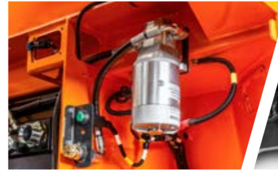
Oil top-off pump (service package)
