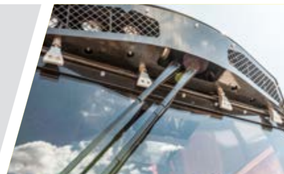
Air-window cleaning system
