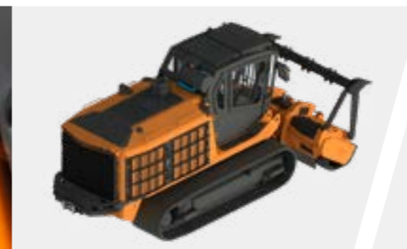
Forestry protections kit (Cabin side windows protection grids + Engine bay doors protections)
