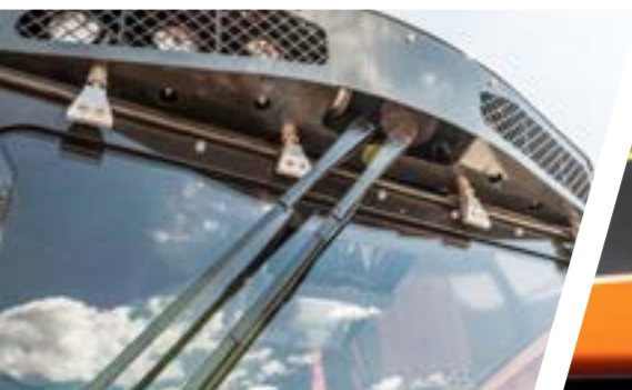
Air-window cleaning system
