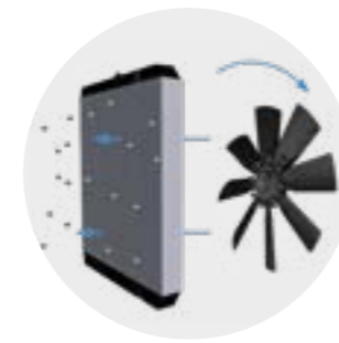
A reversible fan maximizes radiator efficiency (4)
