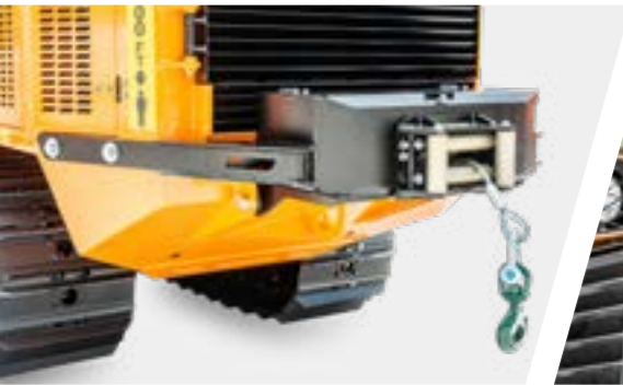
Rear winch - rated towing capacity: 6t
