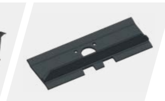
700 mm steel track pads - single grouser
