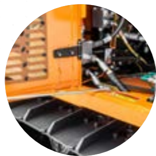
The large rear doors have safety catches (2)
