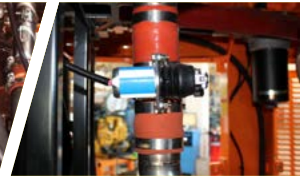
Air shut-off system
