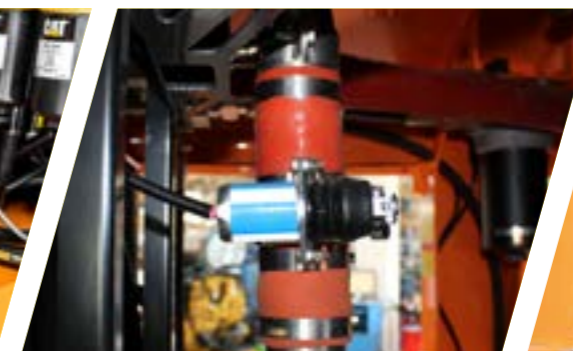
Air shut-off system
