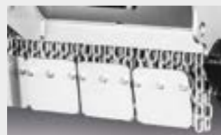
Bolt-on chain's protection plates
