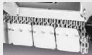
Bolt-on chain's protection plates
