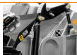
Depth Indicator for precise depth control
