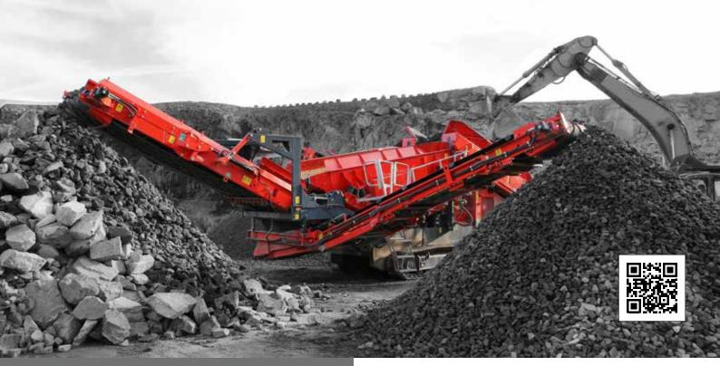
The Finlay® 883+ triple shaft mobile scalping screener is ideal for working in dry and sticky applications including quarry, mining, sand, gravel, construction and demolition debris and recycling applications. The heart of this new model is the new triple shaft screenbox, featuring two "true" full size  $4.8 \times 1.53$ m (16'  $\times 5$ ') screening decks.
