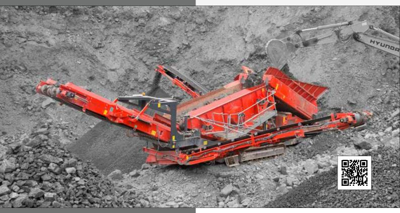
The Finlay<sup>®</sup> 883+ mobile scalping screener has been developed as a high capacity and versatile heavy duty screener to work in primary and secondary screening applications such as quarry and mining, iron ore, construction demolition waste, sand, gravel, compost, top soil and coal.
