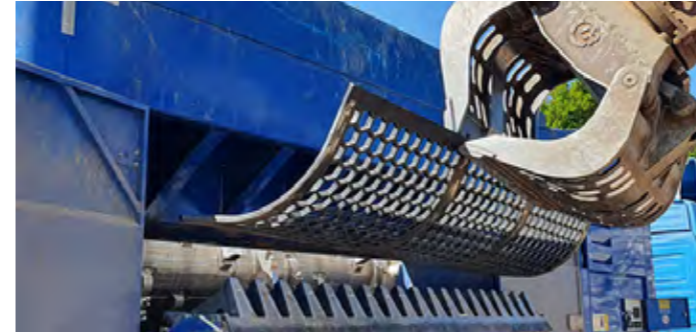
Definition of the final grain via screen baskets and cutting gap
