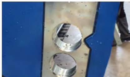
Adjustable cutting gap for final grain size (also Z 50)
