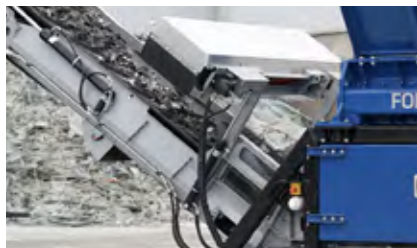
Hydraulically adjustable magnet (also F 38)
