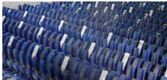
Star screen deck version in durable PU-material (optional)
