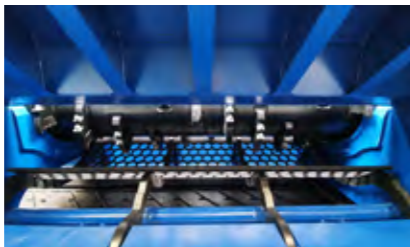
Insensitive to disruptive material due to reversing rotor (also Z 50)
