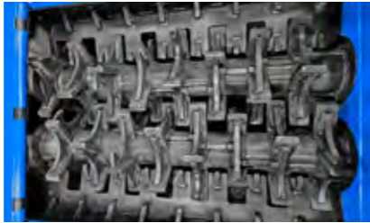
Individually adjustable shaft speeds (also F 25)
